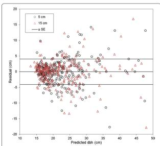
**Fig. 6** Residuals for the stem shape model. Residuals for the prediction of DBH from diameter measurements (Eq. 1). Measurement heights above ground are 5 cm (*black circle*) and 15 cm (*red triangle*). The standard error (SE) is marked by the horizontal *black lines*
