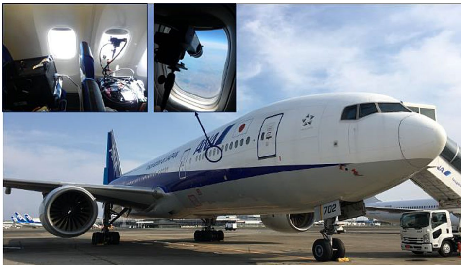
Fig. 3 The GOBLEU instrument suite onboard the ANA aircraft. The instruments are seated on cabin seats (top left panel), targeting the input optics to slant-view through the cabin window (top right panel)
